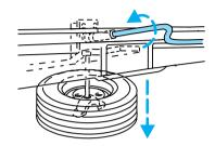
4. Turn the handle counterclockwise until tire is lowered to the ground and the cable is slightly slack.
